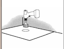
**2** Create a hole in this section of the floor, 140mm to 150mm diameter.
