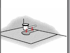
2 Create a trench in the floor to hold the drain pipe and the gully (the gully is 90mm deep). Ideally the hole for the gully should be 130 to 150mm diameter.
