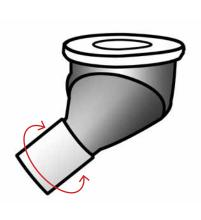
Adjust the angle of the gully to meet the outlet pipe ensuring that is at a suitable angle to drain the water. Then solvent weld the BS40mm pipe to the gully. Replace the boards ensuring that the drain is aligned with the hole. Then follow steps 5-8.
