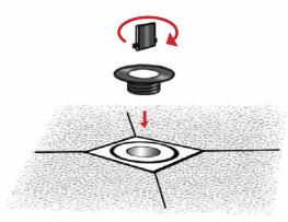
Screw the flange ring into gully underneath ensuring it is flush with the black plastic surround. Use the red "key" to tighten it so that the rubber ring on the gully forms a seal with the steel plate on the backside of the tray. Do not use silicone or any other sealants here.
