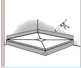
Fix the Shower tray to the plinth using Marmox MSP360 ensuring the waterproof fleece is also fixed flat on the exposed plinth and up against the adjacent wall. When folding the fleece upwards, place a bead of MSP360 between the fleece and the edge of the shower tray. Then follow steps 5 and 7.
