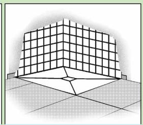
**8** Marmox Multiboard can be used to raise the surrounding floor height and provide a decoupling, waterproof layer. Tile the surrounding floor and walls on top of the surplus fleece attached to the underside of the tray. Put the grate into place and the shower tray is now ready to use.
