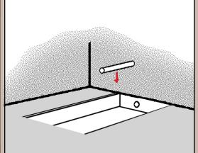
**3** Cut away an area of the boards large enough to span the joists, so that it will be supported when replaced. With the boards removed, install the waste pipe.
