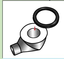
**5** Place the black rubber ring around the outside edge of the gully. This needs to make contact with the steel plate on the back side of the tray.
