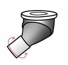
Adjust the angle of the gully to meet the outlet pipe ensuring that is at a suitable angle to drain the water. Then solvent weld the BS40mm pipe to the gully.
