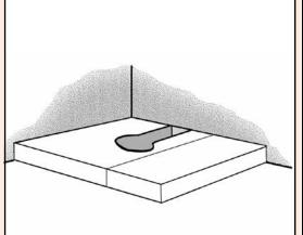
A hole for the drain and drain pipe should now be cut into the XPS. Ensure the hole is just slightly bigger than the drain (approx. 140mm diameter) the fix to the floor and seal to the wall with MSP360.
