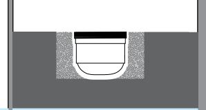
4 Loosely in-fill around the drain and pipe to support the underside of the tray. Do not completely rigidly fix the gully into place and ensure there is a small gap to allow the rubber ring to be fitted. Then follow steps 5-8.
