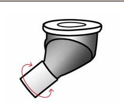
Adjust the angle of the gully to meet the outlet pipe. Then solvent weld the BS40mm pipe to the gully.
