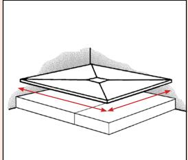
The Marmox Plinth is a solid section of rigid waterproof XPS supplied in sections of 1000 x 1500 x 100mm. These pieces should be cut or combined together to create a solid stable base with the same dimensions of the Decotray.
