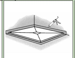
Fix the Shower tray to the floor using Marmox MSP360 ensuring the waterproof fleece is also fixed flat on the surrounding floor and up against the adjacent wall. When folding the fleece upwards, place a bead of MSP360 between the fleece and the edge of the shower tray.
